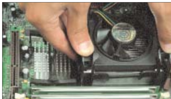
Step 5a: Use both hands if necessary to get a good grip on the heatsink while detaching it
