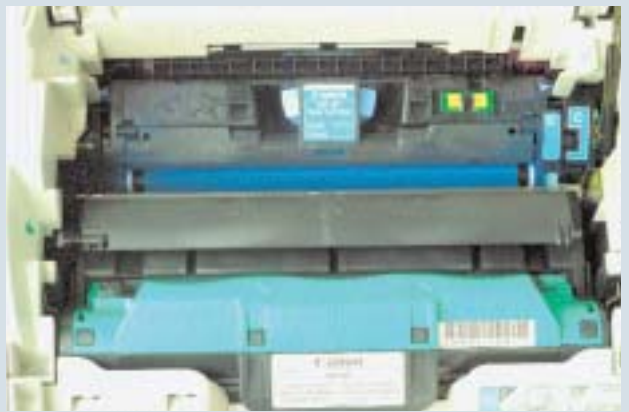
Shown above is the drum cartridge that holds the photoreceptor drum and corona wires. On the opposite side is the Cyan toner cartridge, which also holds the toner developer and toner hopper.
