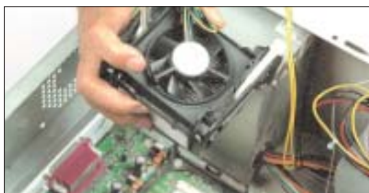
Step 5b: Lift the heatsink clear outside the cabinet, before going for the processor
