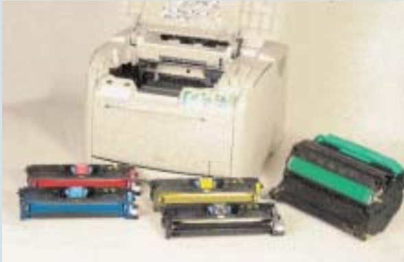
Shown here are the four toner cartridges that are responsible for the colour, and the toner drum with Photoreceptor roller (green roller).
