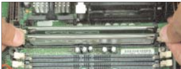
Step 10a: Press firmly on the white clips with your fingers to release the RAM
