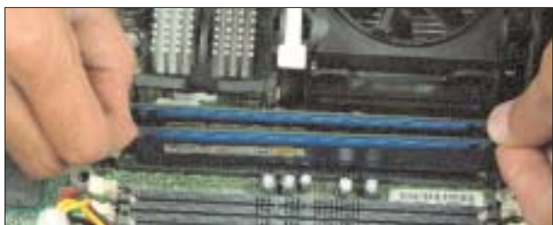
Step 10b: To insert the RAM module easily, hold it at an angle above the slot
