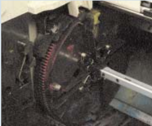
This figure shows the holder, where the toner cartridge are seated. The gear, which is motor driven, helps in rotating the toner cartridge.
