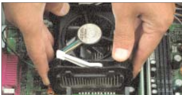
Step 9: Lower the new heatsink slowly, till it sits snugly above the processor
