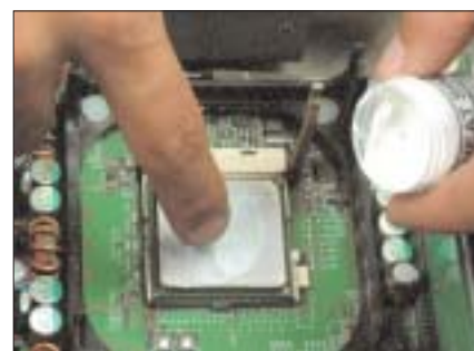
Step 7: Apply the thermal paste gently to form a thin film on the processor's surface
